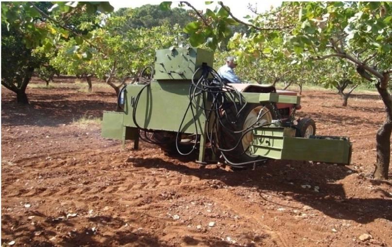
**Fig. 2. Orchard tests with body shaker**
